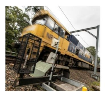
Effective rail lubrication substantially reduces noise from trains along curved track. Transport for NSW has shown through trials that modern, electronic lubricators are more effective and efficient than older mechanical lubricators. We have introduced a new standard for lubrication across the network and we are working with Sydney Trains to implement this standard.
