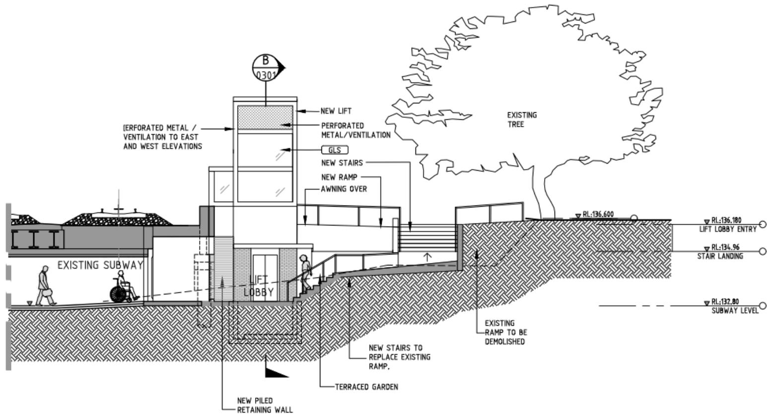
**Figure 3.5 Indicative elevation of the Proposal looking south showing the western lift arrangement**
