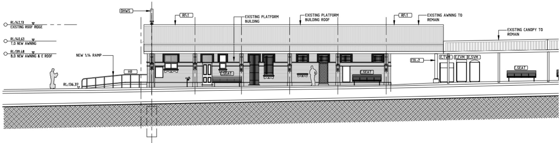
**Figure 3.3 Indicative elevation of the Proposal looking west showing the southern end of the platform and station building**
