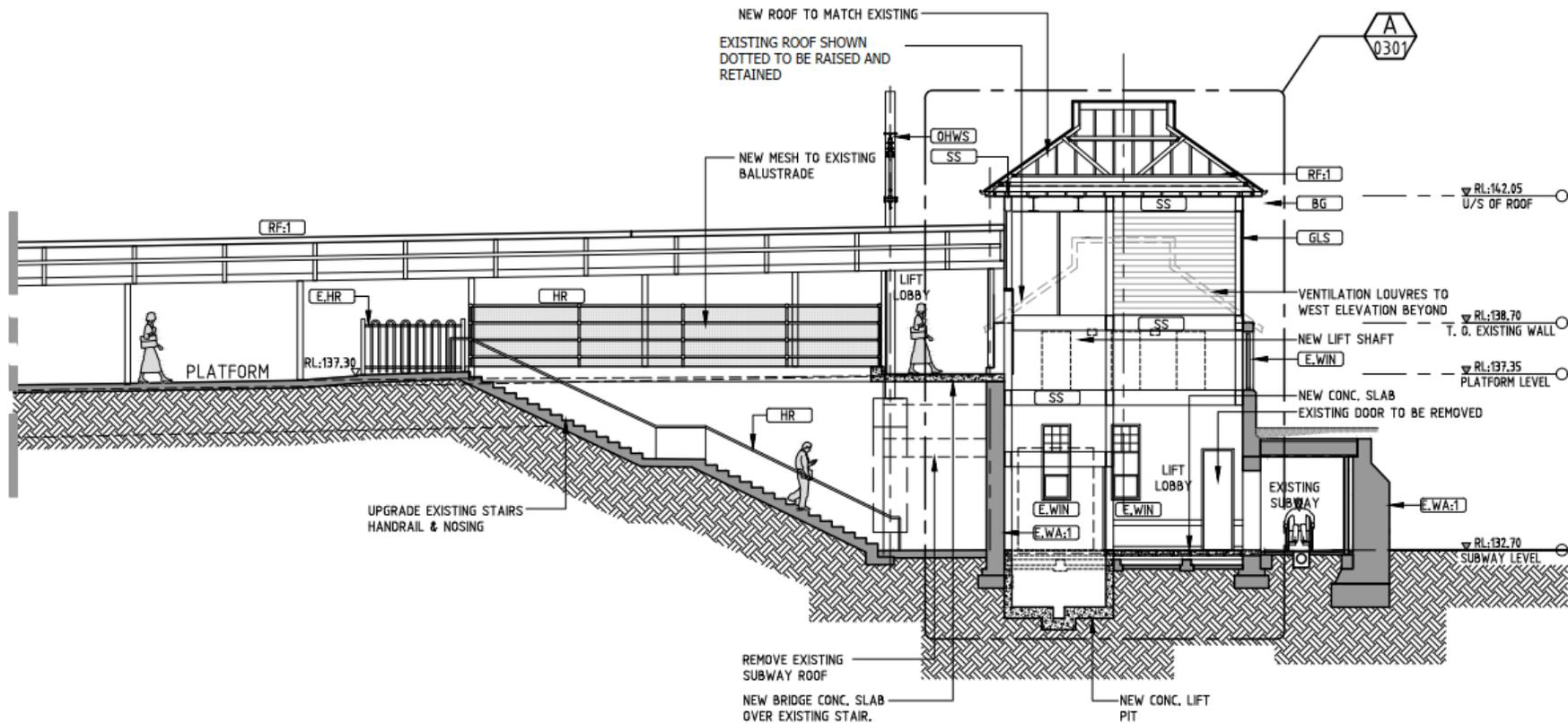
**Figure 3.4 Indicative elevation of the Proposal showing the proposed lift at the northern end of the platform**
