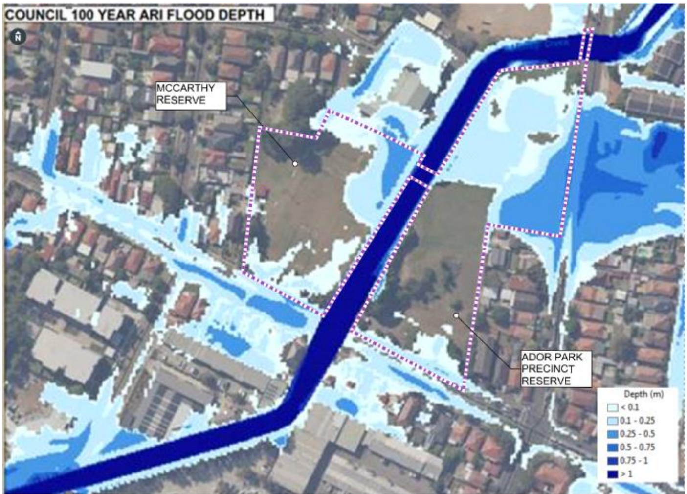
Figure 6-10: McCarthy Reserve/Ador Park Precinct Bayside Council flood model for present day 1% AEP flood patterns (provided by Bayside Council, April 2019)
