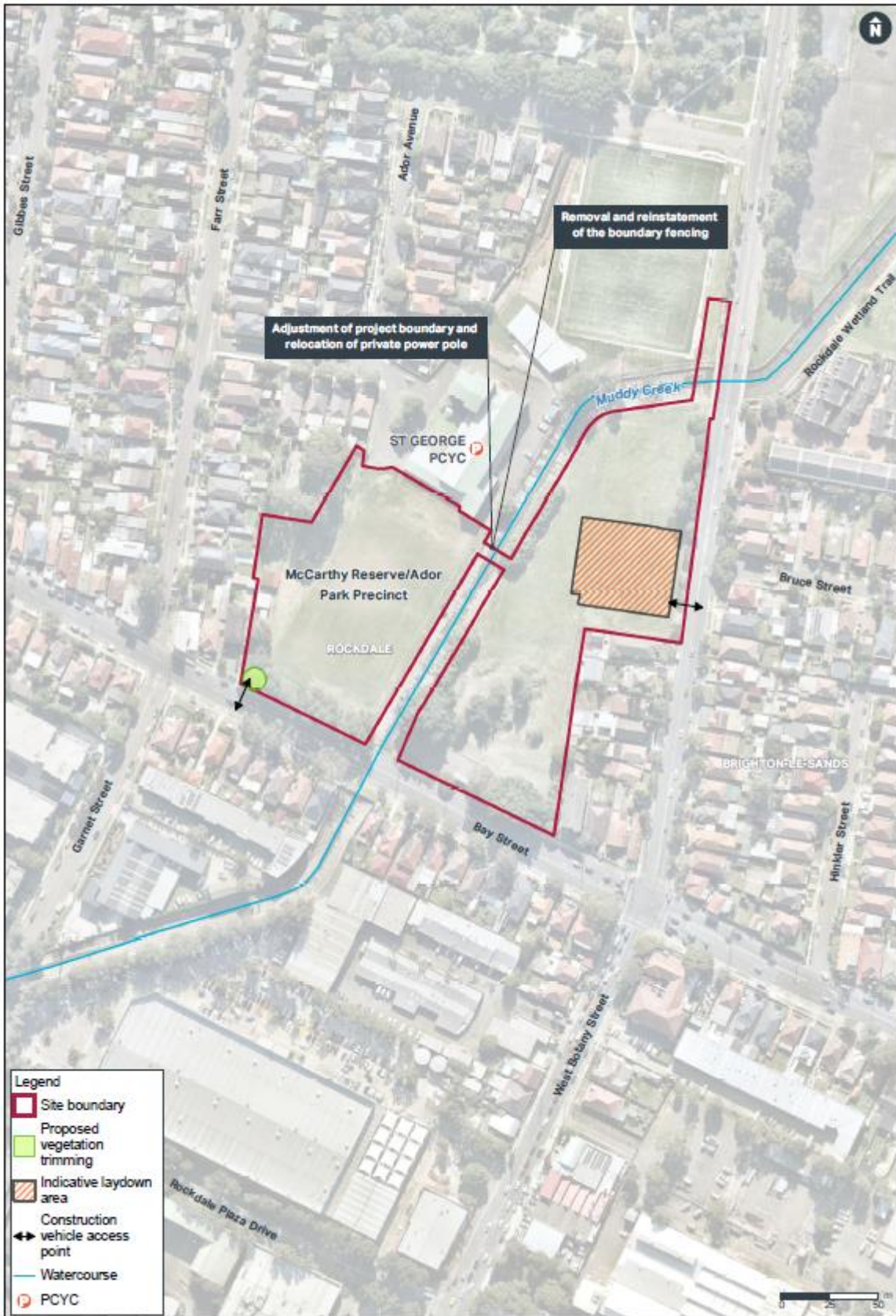
Figure 1-2: The proposed modifications and project construction site layout at McCarthy Reserve/Ador Park Precinct
