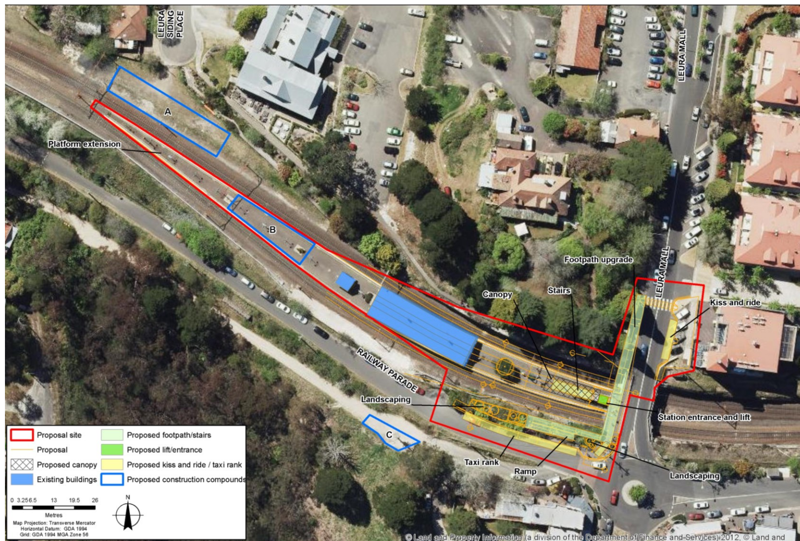
Figure 9 General layout of key elements of the Proposal (indicative only, subject to detailed design)
